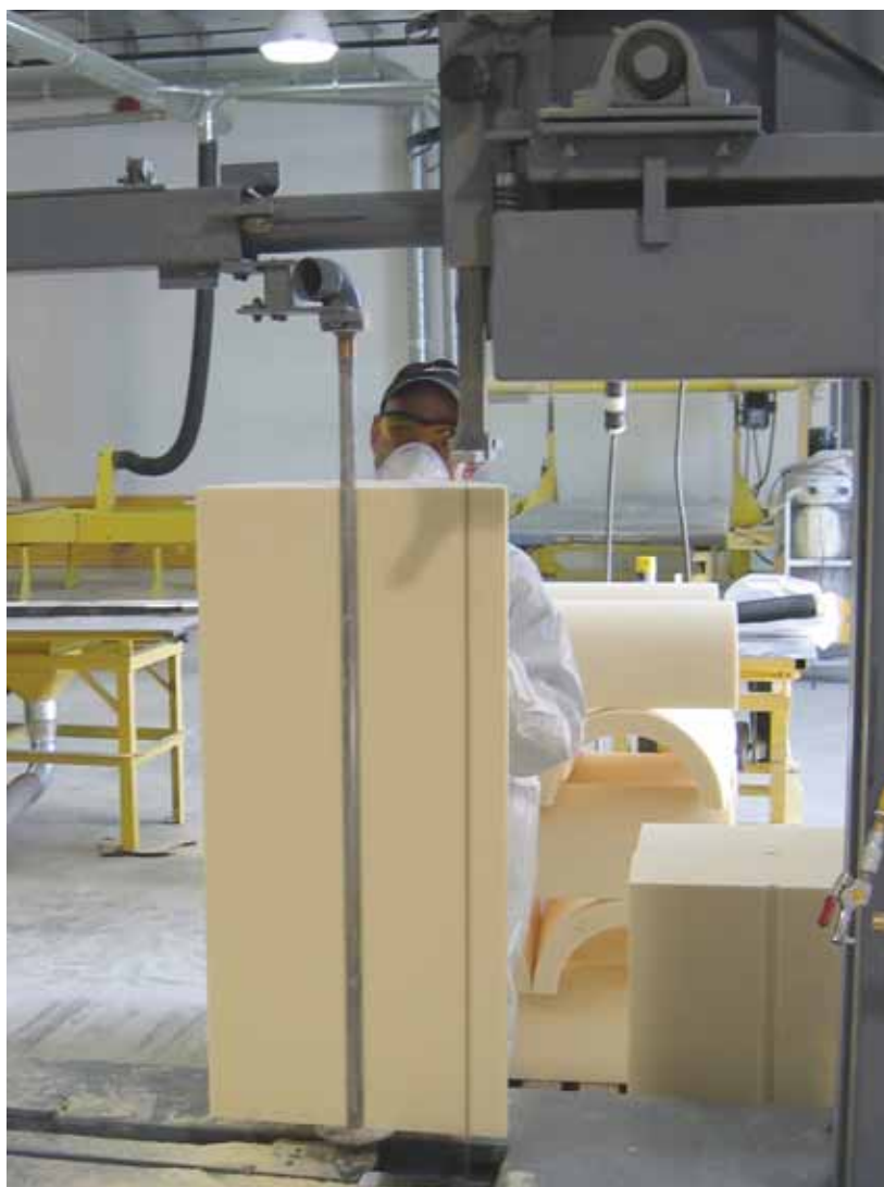
Cutting Trymer ® pipe covering at Polybrand.
