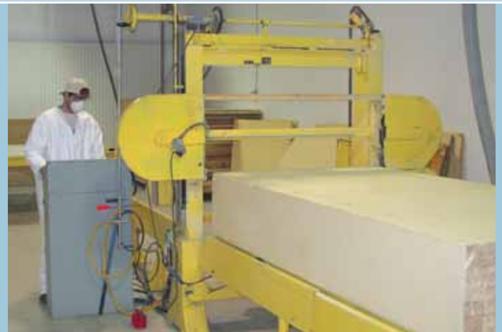
Cutting sheets of Elfoam® on Polybrand's slabbing saw.
